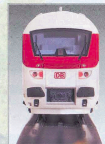
When operated control car last, dual red marker lights shine.
