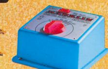
6731 DC control box for 220 volt Output 12 voltampere · track voltage (DC) adjustable between approx. 2 and 8 volt · Pole-changing switch for setting direction · Lighting voltage (AC) 10 volt · Blue plastic housing Weight 2.64 lbs · Dimensions
