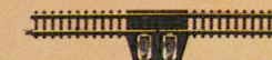
8598 Insulating track section, straight. With terminals. The rail nearest the terminals is interrupted at the centre. Length 4 3/8".
